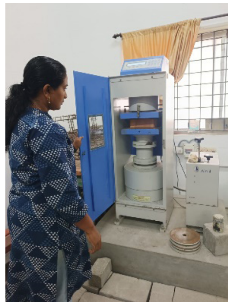
Figure 3: Compressive strength testing of mini compressed earth blocks
