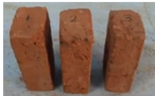
Figure 2: Compressed stabilized earth blocks
